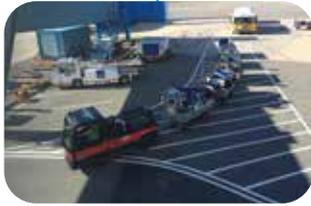
The Speed Control System is a light system: one module per motorized asset and detection beacons. When the vehicle gets closer to a restricted speed area, it automatically and smoothly slows down. Out of these areas, the speed is released to normal state to ensure productivity.
